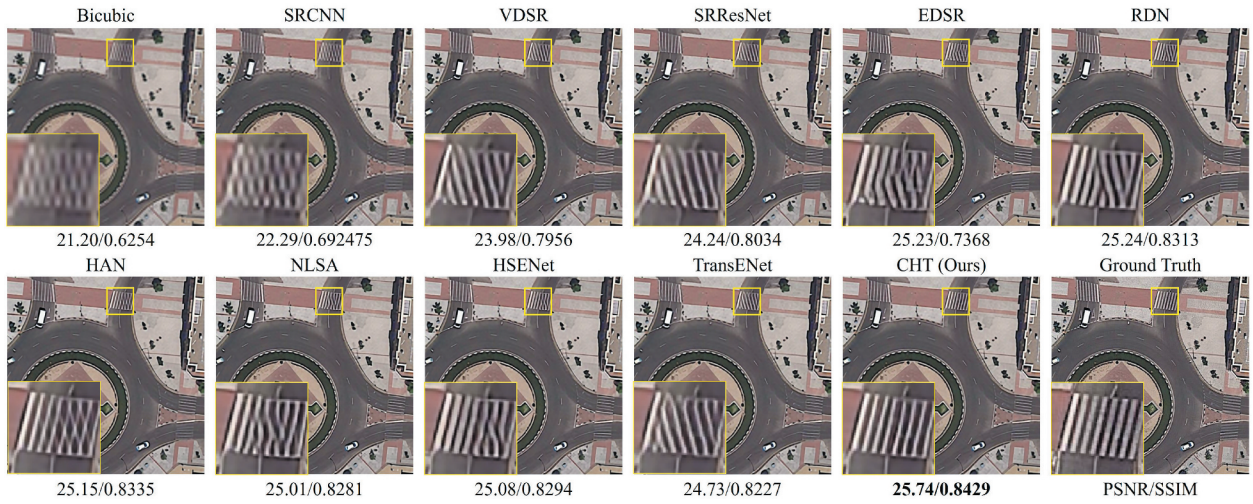
Figure 6. Visual comparisons on the DOTA v1.0 test set, where the selected scenes contain rich cross-scale local details (e.g., cross-scale ground lines). The best PSNR/SSIM is shown in bold . Zoom in for better comparison.
